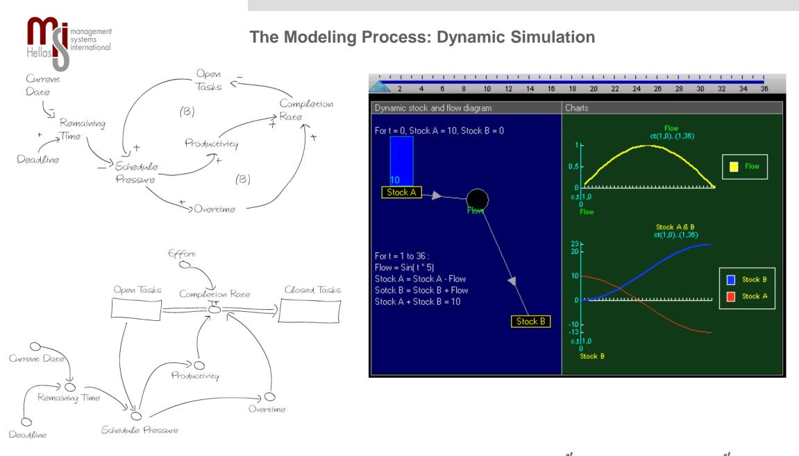
Equations that change the two stocks via the flow are: Stock  $A = \int_0^t -F \log dt$  Stock  $B = \int_0^t F \log dt$
